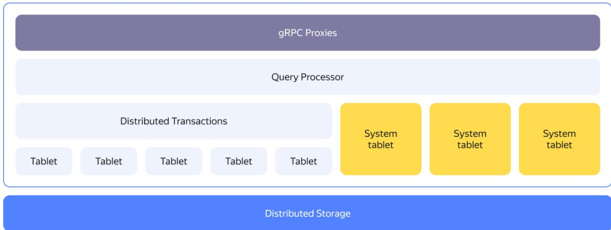
YDB clusters typically run on commodity hardware with a shared-nothing architecture. From a bird's eye view, YDB exhibits a layered architecture. The compute and storage layers are disaggregated; they can either run on separate sets of nodes or be co-located.
