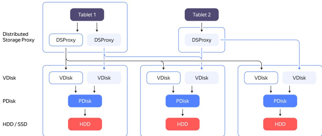
YDB doesn't rely on any third-party filesystem. It stores data by directly working with disk drives as block devices. All major disk kinds are supported: NVMe, SSD, or HDD. The PDisk component is responsible for working with a specific block device. The abstraction layer above PDisk is called VDisk. There is a special component called DSProxy between a tablet and VDisk. DSProxy analyzes disk availability and characteristics and chooses which disks will handle a request and which won't.
